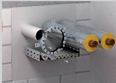
Mount pipe sleeves for combustible pipes on both sides of the wall.
