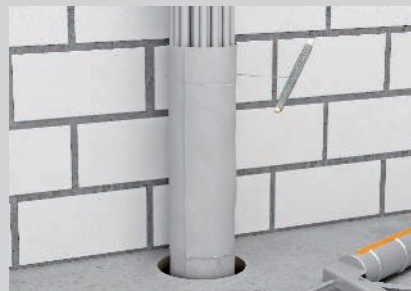
Fixing of the bandage using winding wire.
