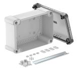
Junction box with hat profile rail for the connection of cables and lines indoors and in outdoor areas. Rectangular design without entries. Suitable for wall and ceiling mounting with the option to fasten outside, inside or to mount via the corner domes. Particularly impact resistant with IK08. Transparent cover with quick lock, sealable. Made from halogen-free and UV-resistant materials.
