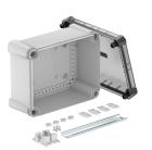
Junction box with hat profile rail for the connection of cables and lines indoors and in outdoor areas. Rectangular design without entries. Suitable for wall and ceiling mounting with the option to fasten outside, inside or to mount via the corner domes. Particularly impact resistant with IK09. Transparent cover with quick lock, sealable. Made from halogen-free and UV-resistant materials.
