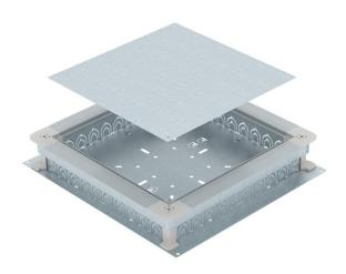
Underfloor junction and branch box for 10 installation pipes on each side (M20 or M32) with sheet steel side walls. To mount installation units in the mounting lid (to be ordered separately). Height can be infinitely adjusted to the nominal screed height (rapid adjustment possible) and the screed can be worked flush to the screed scraping edge. With noise decoupling option after screed laying and can be used with system accessories, also for heavy-duty application.
