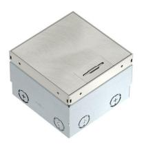
Square floor socket for use in dry-care cavity and screed floors in indoor areas. Installation housing with pre-marked insertion openings for pipes (M20/M25). Cover adjustable to top edge of floor covering using four height-adjustment supports. The minimum installation depth is 100 mm, the height-adjustment range is +35 mm.
