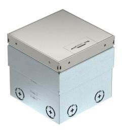
Square floor socket for use in dry-care cavity and screed floors in indoor areas. Installation housing with pre-marked insertion openings for pipes (M20/M25). Cover adjustable to top edge of floor covering using four height-adjustment supports. The minimum installation depth is 100 mm, the height-adjustment range is +35 mm
