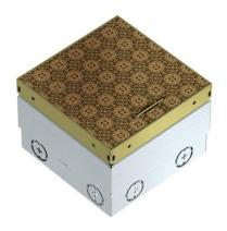
Square floor socket for use in dry-care cavity and screed floors. Installation housing with pre-marked insertion openings for pipes (M20/M25). Cover adjustable to top edge of floor covering using four height-adjustment supports. The minimum installation depth is 100 mm, the height-adjustment range is +35 mm.
