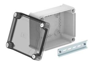
Closed junction box for the connection of cables and lines indoors and in protected outdoor areas. Rectangular design without entries. Suitable for wall and ceiling mounting and on mounting panels. With the option to fasten inside and to mount via the corner domes. High, transparent cover with quick lock, sealable. Made from halogen-free and UV-stabilized materials.
