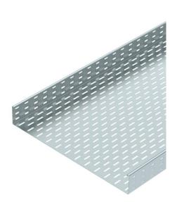
SKS 85 = heavy-duty cable tray system with 85 mm side height. FS version includes connector, type RLVL 85. Magnetic shield insulation without cover 20 dB, with cover 50 dB.
