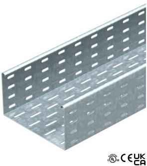
SKS 110 = heavy-duty cable tray system with 110 mm side height. FS version includes connector, type RLVL 110. Magnetic shield insulation without cover 20 dB, with cover 50 dB.
