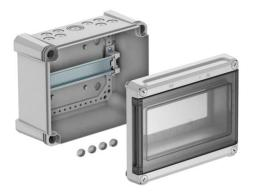
Small distributor for surface mounting, for the current sub-distribution in interior and exterior areas, according to IEC 439-3. With pre-mounted 35 mm hat profile rail. IP66 protection type and IK08 protection rating. Transparent cover to screw on, with cut-out. Including 4 screw cover caps.
