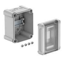
Small distributor for surface mounting, for the current sub-distribution in interior and exterior areas, according to IEC 439-3. With pre-mounted 35 mm hat profile rail. IP66 protection type and IK08 protection rating. Transparent cover to screw on, with cut-out. Including 4 screw cover caps.
