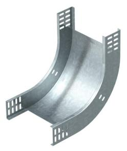
90° rising vertical bend, for all cable tray types of 60 mm side height. The vertical bend is pushed over the end of the cable tray and screwed tight. Fastening materials should be ordered separately.
