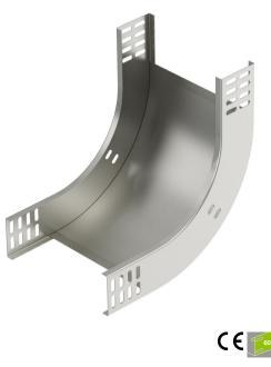
90° rising vertical bend, for all cable tray types of 60 mm side height. The vertical bend is pushed over the end of the cable tray and screwed tight. Fastening materials should be ordered separately.
