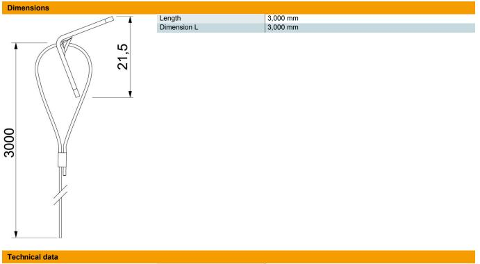
Operating load Cable diameter 45 kg 2 mm
