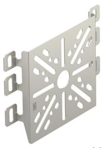
Mounting plate, for fastening on the side rail of cable support systems. Fastening on the side rail of the mesh cable tray is carried out without bolts by bending the lugs. Fastening on the side rail of cable trays or cable ladders is carried out with two truss-head bolts. Type B9/T junction boxes can be mounted very easily by inserting the bolt plug supplied into the centre hole on the mounting plate.
