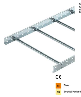
Cable ladder with perforated side rail of side height 75 mm with riveted C profile rungs, open in an upwards direction. Assignment of the rungs on both sides possible using U clamps. Magnetic shield insulation without cover 10 dB, with cover 15 dB.
