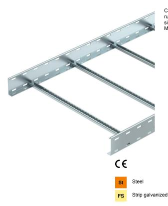
Cable ladder with perforated side rail of side height 100 mm with riveted C profile rungs, open in an upwards direction. Assignment of the rungs on both sides possible using U clamps. Magnetic shield insulation without cover 10 dB, with cover 15 dB.
