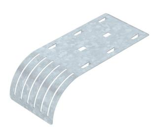
Drop-out plate for mesh cable trays. The exit plate allows compliance with specific bend radii, thus preventing possible cable breaks. Can be mounted in a lengthwise direction and at the side, can also be arranged next to each other for greater widths.
