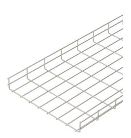
Mesh cable tray made of spot-welded steel wire of side height 55 mm. The grid dimension is 50 x 100 mm. Magnetic shield insulation without cover 15 dB, with cover 25 dB.
