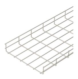
Mesh cable tray made of spot-welded steel wire of side height 55 mm. The grid dimension is 20 x 100 mm in the width 50 mm and 50 x 100 mm in the widths 100-600 mm.
