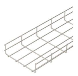
Mesh cable tray made of spot-welded steel wire of side height 55 mm. The grid dimension is 20 x 100 mm in the width 50 mm and 50 x 100 mm in the widths 100-600 mm.
