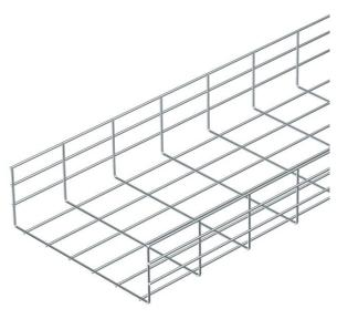
Mesh cable tray made of spot-welded steel wire of side height 105 mm. The grid dimension is 50 x 100 mm.
