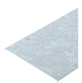
Cover for cable trays and cable ladders with three pairs of turn buckles. Transverse bead from 500 mm width. When using covers outdoors, additional measures against the influence of wind must be taken.
