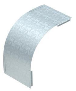
Cover for falling vertical bends of side height 85 mm. The fastening is guaranteed by the overlap of the cable tray covers. The cover can also be fastened using cover clamps.
